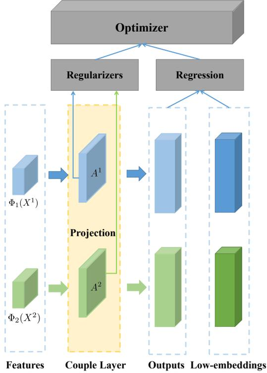
Figure 2. Architecture of the couple layer. It takes two input layers and generates two output layers. Meanwhile it delivers the shrinkage regularizer to the optimizer.
