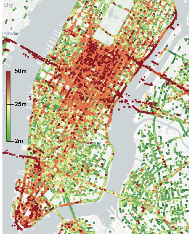
Figure 2. Accuracy of GPS data crowd-sourced from over 250K driving hours in NYC. The percentage of rides that experience GPS errors of 10 meters or more (likely due to urban canyons effects) is 40%, and that of 20 meters or more is 20%.
