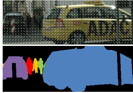
Figure 6. Top: visualization of the Guidance Offsets Table of the Instance Module. Bottom: visualization obtained by coloring with a different color each unique value in the output map.
