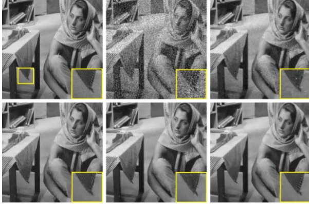
Figure 4. Restoration results of Barbara image (GN + SPN, \alpha = 20 ; \rho = 0.2 ). From left to right and top to bottom: original image, noise image, the reconstructed images by M-BM3D (PSNR = 23.64dB), I1-I0 (PSNR = 29.41dB), WJSR (PSNR = 30.01dB), and our proposed method (PSNR = 31.20dB).
