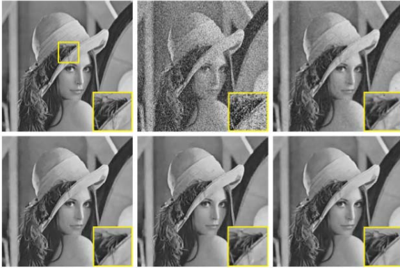
Figure 5. Restoration results of Lena image (GN + SPN, \alpha = 20 ; \rho = 0.2 ). From left to right and top to bottom: original image, noise image, the reconstructed images by M-BM3D (PSNR = 27.61dB), I1-I0 (PSNR = 31.31dB), WJSR (PSNR = 31.69dB), and our proposed method (PSNR = 32.61dB).
