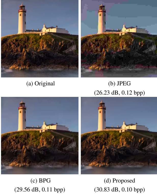
Figure 1. Comparison of image qualities between original, JPEG, BPG, and the proposed. The differences are more evident when zoomed in on the electronic version of this paper.
