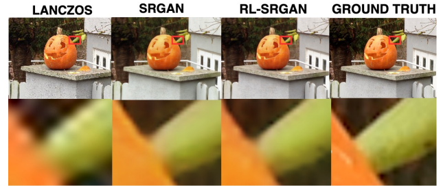
Figure 2: The above figure shows the results for RL-SRGAN compared to SRGAN, LANCZOS, and the original ground truth. As we can see, LANCZOS simply destroys the edges producing artifacts on the global image. Whilst, SRGAN forms noticeable chromatic aberration (i.e transition from orange to yellow color) near the edges. Even though, the RL-SRGAN holds the color uniform with net outline details nearby to the edges; analogous to the original ground truth.
