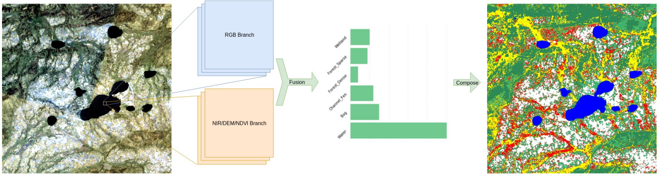
Figure 1. Overview of our proposed ArcticNet. The RGB and NIR/DEM/NDVI branches take their corresponding modality from a same patch. Then, the feature map output by two networks are fused for classification. The semantic label map of the entire area is composed by sliding over the full image.
