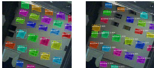
Figure 6. Window labeling (left) and detection results (right) for wrong parameter selection in terms of region proposal threshold filtering, leading to "missing windows"
