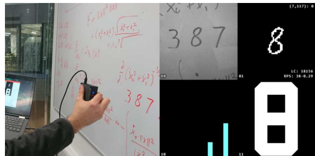
Figure 1. Digit prediction with a CNN from hand-drawn input (left) using inference of a MNIST trained CNN to produce the correct output (bottom-right corner). This demo uses the SCAMP5, a sensor-processor that enables true end-to-end capture and processing with a CNN on its massively parallel pixel-processor array.
