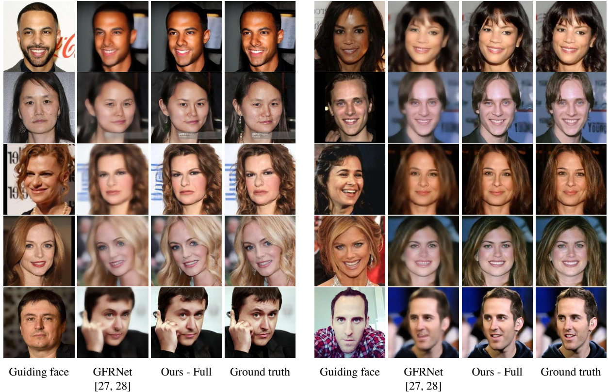
Figure 5: Comparison with state-of-the-art. Our full model GWAInet produces perceptually high quality images while retaining the facial features related with the identity. To obtain the results for GFRNet, their publicly available model is used [27, 28]. [8× upscaling, LR input spatial dimensions 32 × 32]
