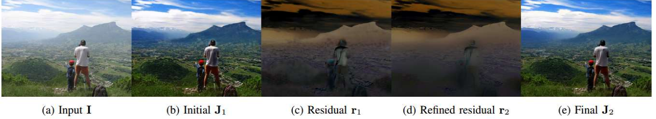
Figure 3: The proposed post-processing module for halo suppression. The initial dehazed image J_1 is the input. We first obtain r_1 via elemental-wise subtraction Elti(I, J_1) . Then refined residual r_2 is obtained by applying guided filtering to r_1 ( I is the guidance). Finally, J_2 is recovered from Elti(I, r_2) .
