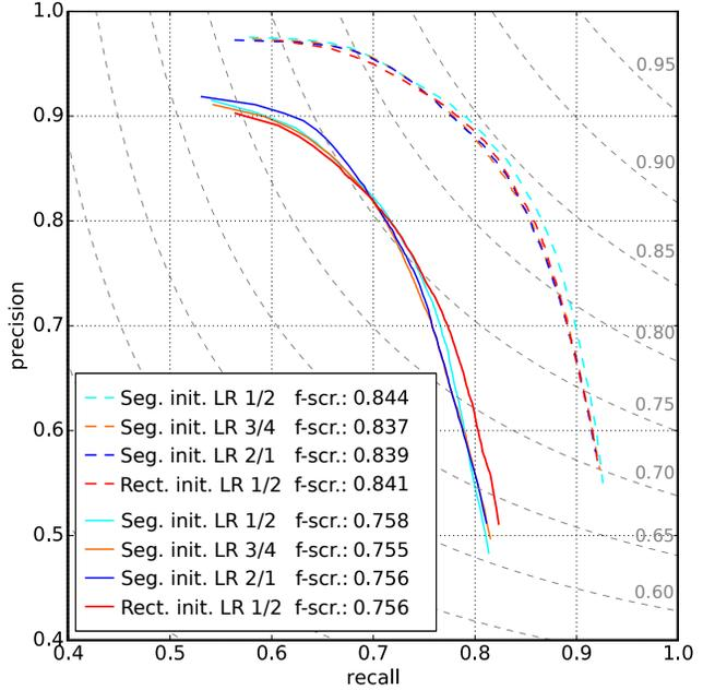
Figure 6. Evaluation of three different detection and segmentation loss ratios (LR) for weakly supervised recursive training [28] (MRCNN recursive) initialized with the instance segmentation labels (seg. init.) created by Algorithm 1. Rect. init. represents the naïve initialization using the entire GT box. Solid curves represent results for an IoU threshold of 0.5 and dashed curves for 0.3.
