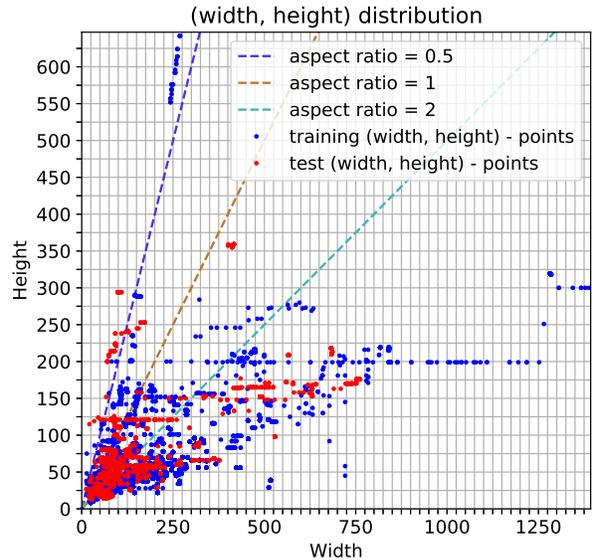
Figure 5. Training and test samples plotted as width/height points and the three RPN anchor aspect ratios depicted as straight lines.
