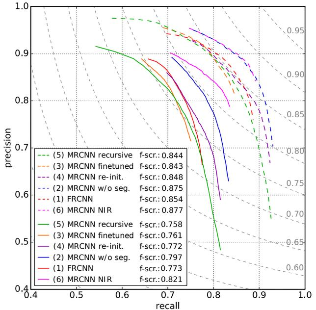
Figure 7. Best results for each experiment represented by precision-recall curves and maximum f-score. Solid curves represent results for an IoU threshold of 0.5 and dashed curves for 0.3. The dashed grey curves show the f-score.
