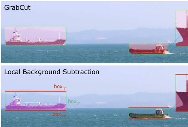
Figure 4. Instance segmentation labels created by GrabCut and Algorithm 1. While GrabCut is prone to produce FP segmentations right above the vessels, Algorithm 1 tends to produce FNs. The depicted boxes correspond to the ones mentioned in Algorithm 1.
