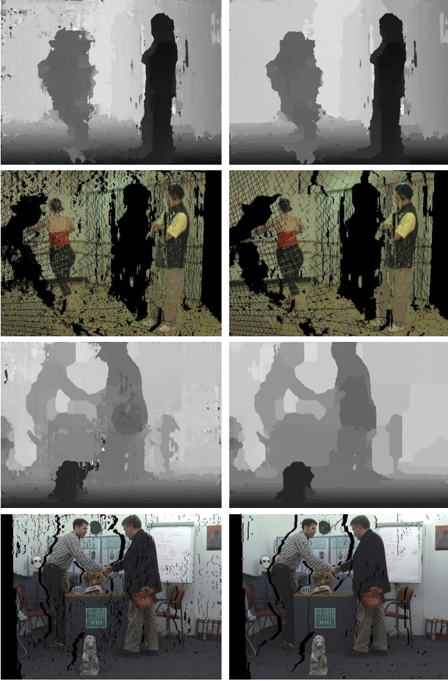
Figure 1. First column: depth maps and corresponding renderings computed without temporal constraints. Second column: depth maps and corresponding renderings with temporal constraints for the ballet [10] and book arrival [11] datasets.
