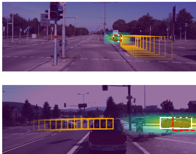
Figure 1. Visualization of past localizations of a tracked vehicle (orange), predicted +1 second future localization (red, dashed), and the true +1 second future localization (white), drawn over the +1 second future frame. The area of confidence is highlighted around the predicted box. Our method predicts the red dashed box as the mean B(t) of a robust 4D probability distribution based on the Huber loss with scale parameter \sigma(t) , given only the sequence of orange bounding boxes as input. This model well captures the potential amount of divergence for different input scenarios. In both instances above, a car is observed traveling through an intersection, but the lateral view (bottom) has a larger spread of possible bounding boxes due to the car speeding up or slowing down.
