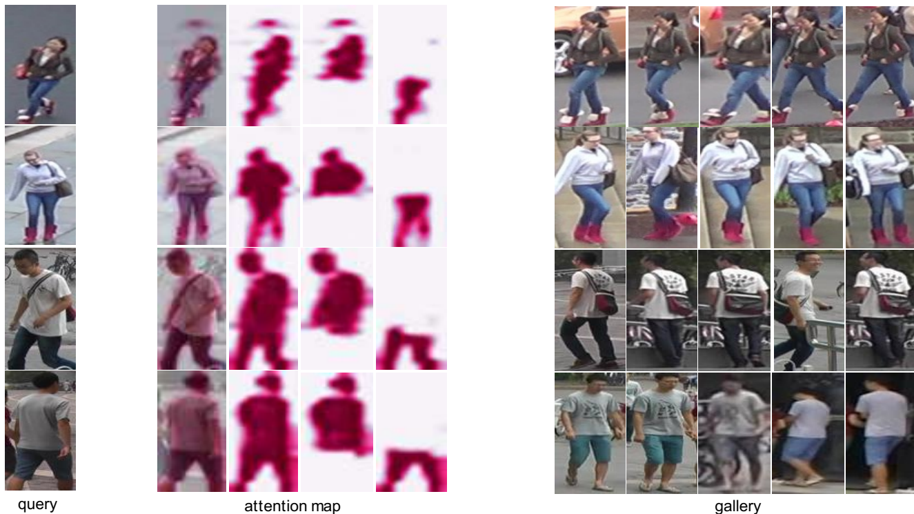
Figure 5. The top-5 ranking list for the query images on Market-1501 and DukeMTMC-reID by MMGA. The retrieved images are from the gallery set and not from the same camera as the query images. The first column is query images. Whole-body attention maps on original images, whole-body attention maps, upper-body attention maps, bottom-body attention maps from our MMGA are in the second to fifth columns. The right side shows the retrieved top-5 ranking images with our proposed MMGA method. All top-5 are correct.
