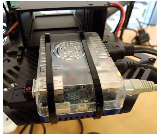
Figure 4: Experimental embedded platform: Odroid-XU4 embedded platform on-board a DJI Matrice 100 UAV
