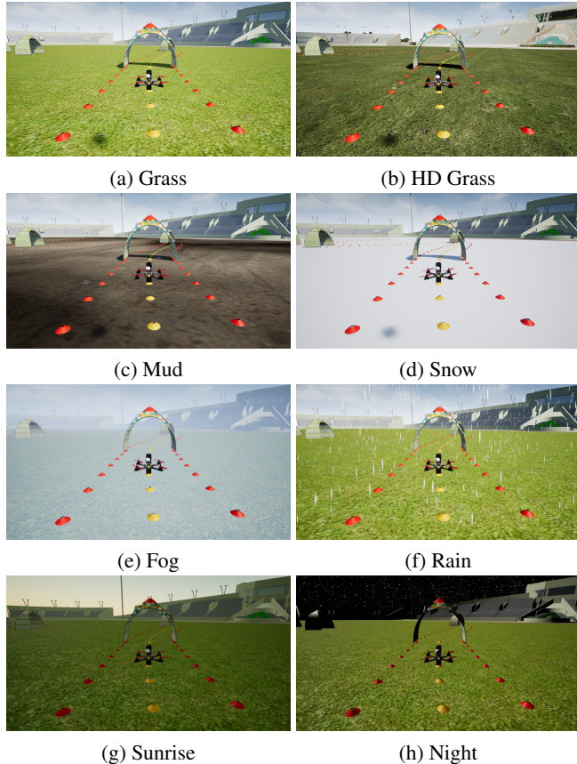
Figure 9: Simulated UAV racing stadium with low and high quality grass textures ( a,b ), different ground materials ( c,d ), different weather conditions ( e,f ) and different lighting conditions ( g,h ).
