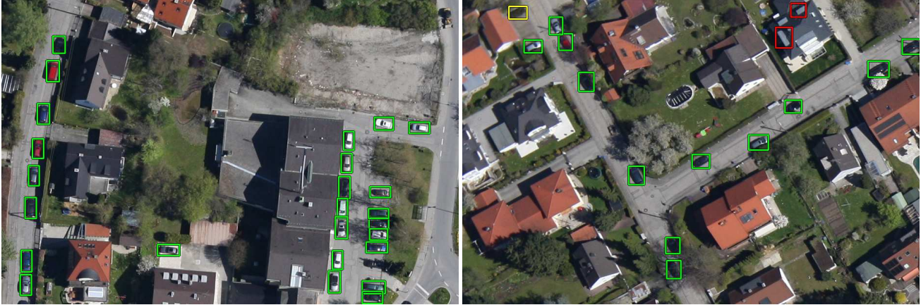
Figure 4: Qualitative results for UAV-Net _{\varphi=0.50} on DLR 3K. A confidence threshold of 50% was used to generate the detections (green boxes = true positives, yellow boxes = false negatives, red boxes = false positives).
