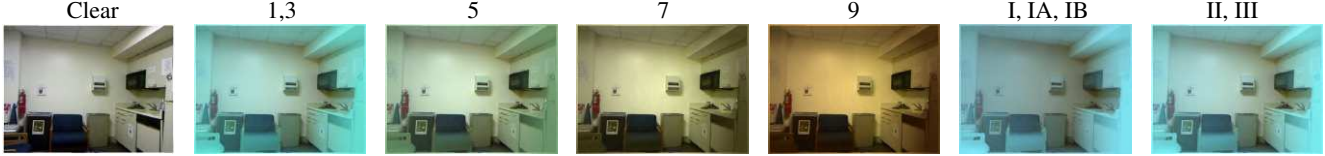
Figure 4. Underwater images synthesized following the approach in [3]. We club similar looking water types into a single class and reduce the total number of classes from 10 to 6 in order to boost the performance of our nuisance classifier.
