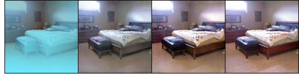
(a) From left to right - Input image, output of vanilla U-Net, output of U-Net with adversarial loss, ground truth image.
