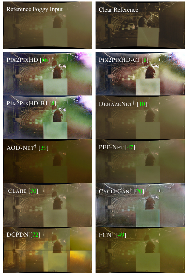
Figure 1: Example image de-hazing results based on our introduced benchmark dataset. It enables evaluating the system performance based on calibrated reflective targets and assessing the contrast enhancement in depth for a challenging illumination setting in different fog densities.
