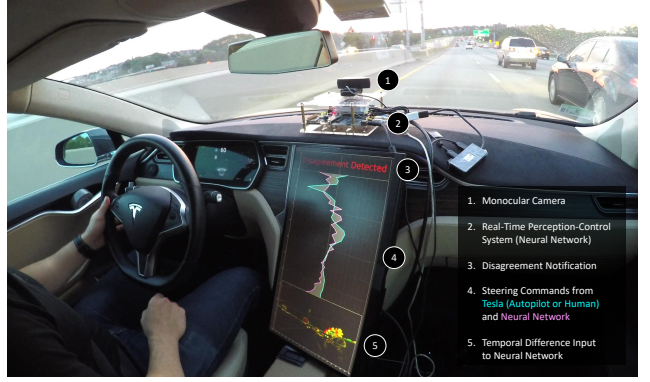
Figure 6: Implementation and evaluation of the system presented in this paper. The primary perception-control system is Tesla Autopilot. The secondary perception-control system is an end-to-end neural network. We equipped a Tesla Model S vehicle with a monocular camera, an NVIDIA Jetson TX2, and an LCD display that shows the steering commands from both systems, the temporal difference input to the neural network, and (in red text) a notice to the driver when a disagreement is detected.
