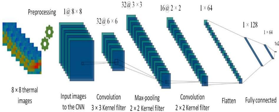
Figure 6. A structural diagram of the proposed 2-D CNN that used to classify captured thermal images into occurrence or non occurrence of convulsive movements.
