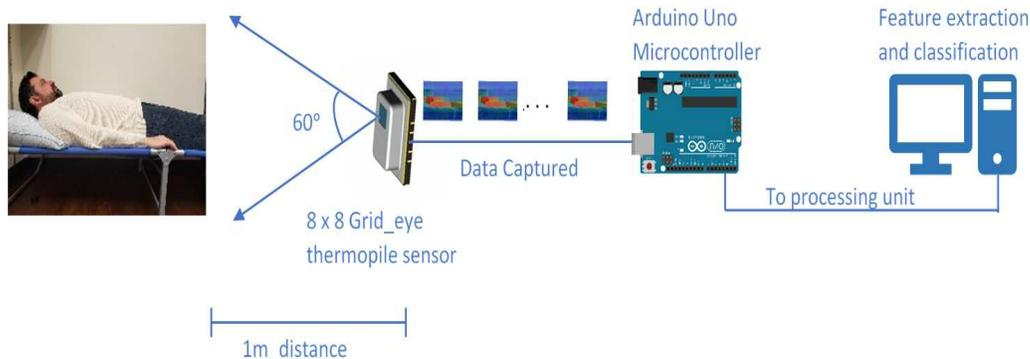
Figure 1. The proposed system consists of a thermopile sensor array, Arduino Uno micro controller, and a processing unit for extracting and classifying data.
