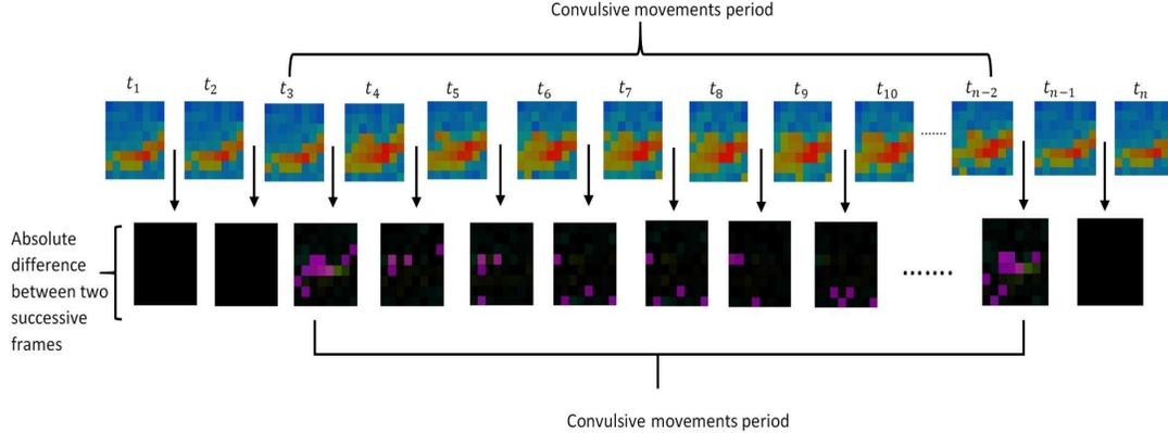
Figure 5. An absolute difference between two consecutive thermal images that captured using an  $(8 \times 8)$  thermopile sensor array.
