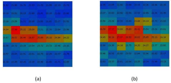
Figure 4. a) A thermal image with corresponding temperature values captured by an  $(8 \times 8)$  sensor array due to no movement (sleep mode). b) A thermal image with corresponding temperature values captured by an  $(8 \times 8)$  sensor array due to convulsive movement.
