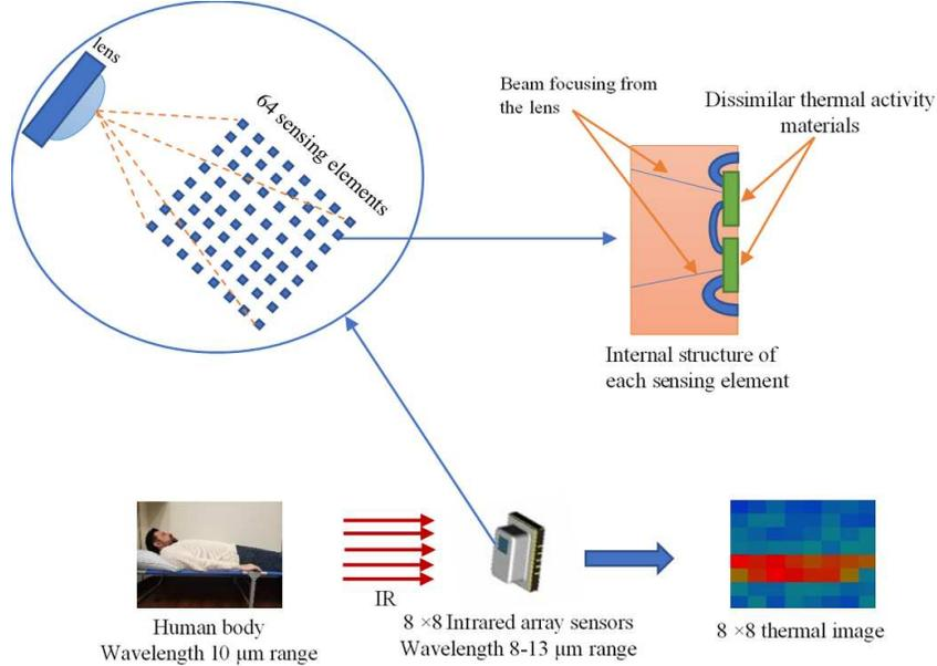
Figure 2. The thermopile sensors that generate a thermal image from the infrared radiation displayed as a matrix.
