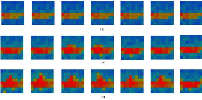
Figure 3. a) A sequence of frames captured by an  $(8 \times 8)$  sensor array due to no movement (sleep mode). b) A sequence of frames captured by an  $(8 \times 8)$  sensor array due to normal movements. c) A sequence of frames captured by an  $(8 \times 8)$  sensor array due to convulsive movements.
