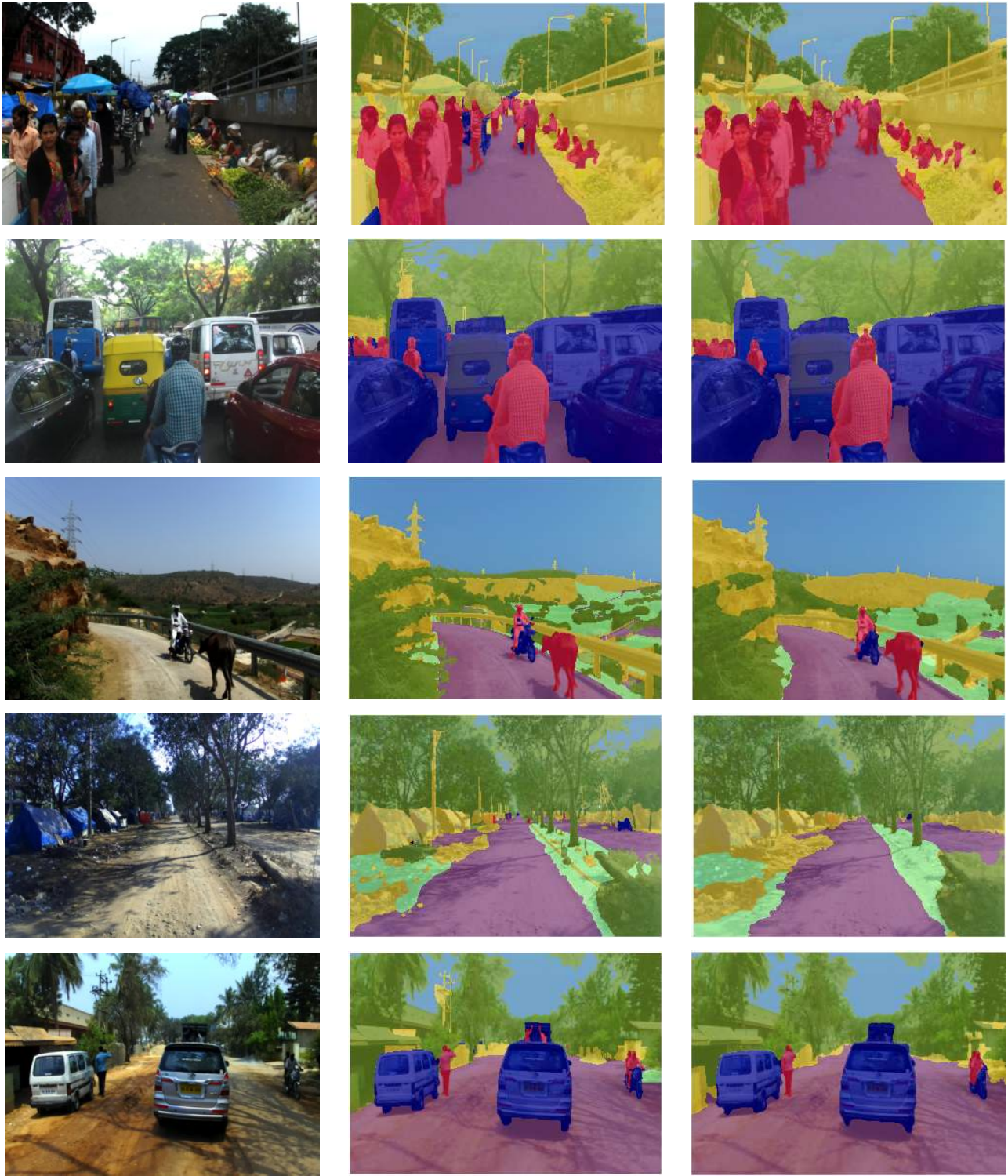
Figure 7: Result of semantic segmentation on IDD Lite validation dataset with proposed architecture. First column shows the input images depicting different scenarios from unstructured environment. Second and third column shows the ground truth and predicted segmentation map respectively where different colours signify different classes.
