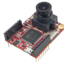
Figure 2. Deployment platform for the proposed solution. On a microcontroller platform (OpenMV Cam M7), we deploy a compact architecture made of about 100k parameters.
