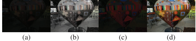
Figure 2. Decomposing an image into lightness and color components. (a) Input low-light image. (b) Lightness enhancement only using CWAN_L . (c) Color enhancement only using CWAN_{AB} . (d) The enhanced image from the proposed CWAN model.
