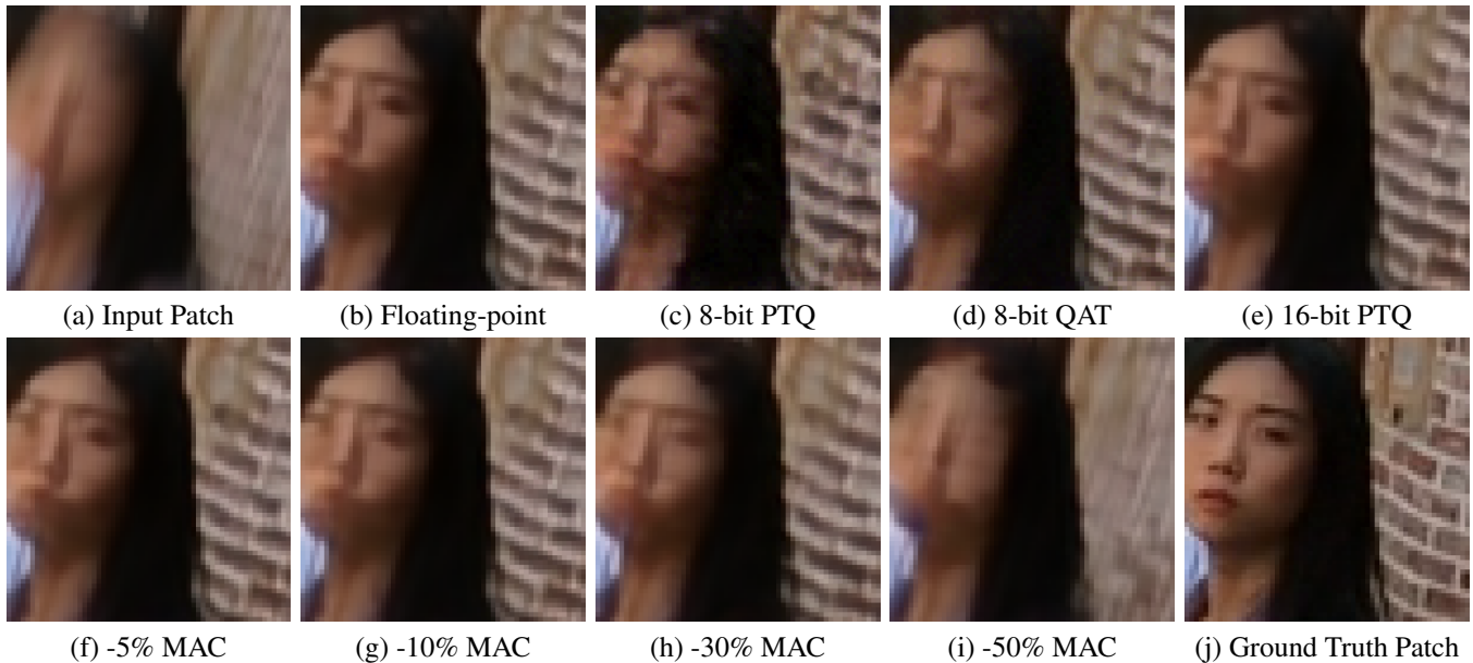
Figure 3. Visual results of UNet-ResizeBilinear-PRelu with network quantization and pruning. (c)(d)(e) represent different quantization settings as in Table 4. (e)(f)(g)(h) show the results of pruning given different MAC reduction targets. The patch is cropped from 000/00000039.png in REDS validation set
