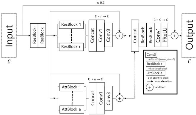
Figure 3. The architecture of Attention Via Concatenation block (AVCblock).
