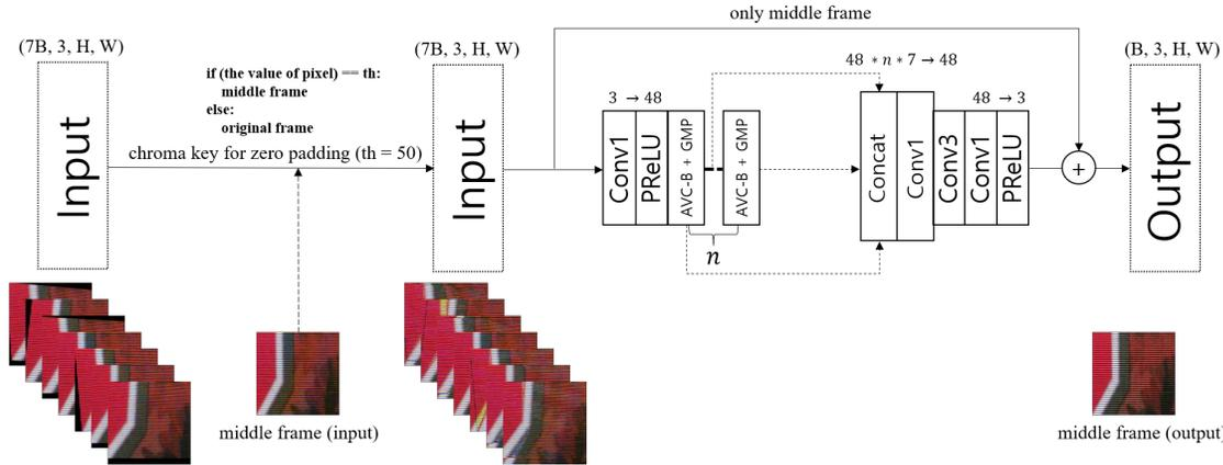
Figure 6. The architecture of C3Net-Burst.
