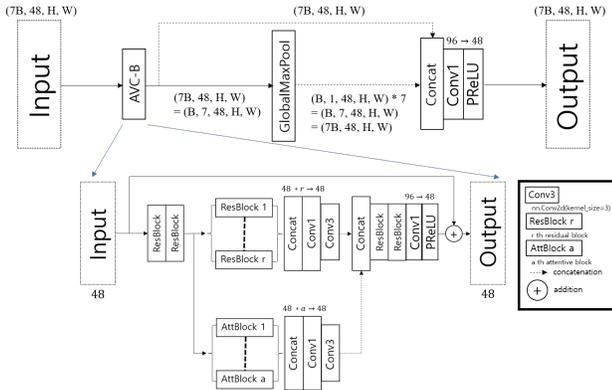
Figure 7. The architecture of AVC-Burst block with global max-pooling (AVC-B + GMP block).
