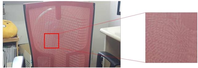
Figure 1. Moiré patterns made by a striped backrest of a chair and a rotating fan (shot with Galaxy S6).
