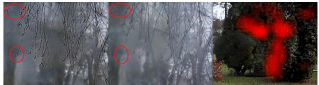
Figure 4: Left: example output image w/o deformable convolution. Middle: example output image with deformable convolution. Right: example output image w/o deformable convolution that contains artifacts.
