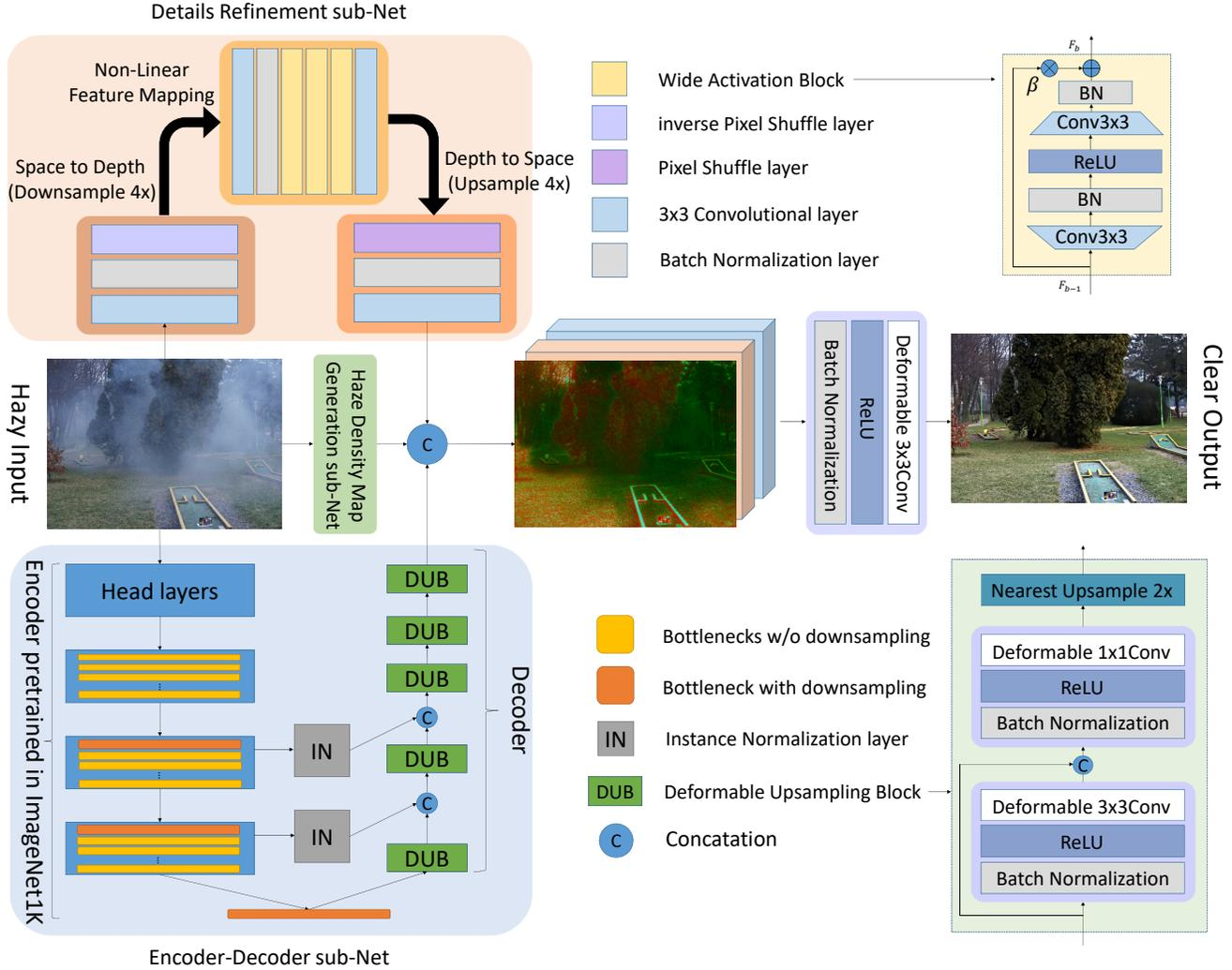
Figure 1: The architecture of the proposed Trident Dehazing Network (TDN), the Details Refinement sub-Net (DRN) and the Encoder-Decoder sub-Net (EDN).  $\oplus$  represents tensor addition and  $\otimes$  represents tensor multiplication respectively. TDN consists of three sub-nets: EDN, DRN and HDMGN. The haze density maps and intermediate feature maps output by three sub-nets are then concatenated and fed into the tail deformable [38] convolution block to get the clear output.
