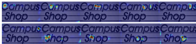
Figure 7: The 2D attention maps on a multi-line example. The 2D attention follows the first text line and then moves to the next line.
