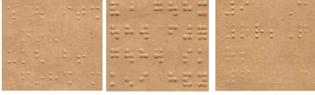
(a) Tiny Braille dots (b) Thick dots (c) Erased dots
