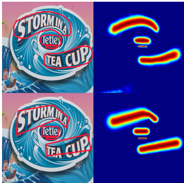
Figure 1. Polygonal text annotations of curved text in images are often so imprecise (bottom left) that heat maps (bottom right), computed as an intermediate step to interpret the text, yield inaccurate results. The proposed UHT method computes and interprets deep learned heat maps (top right) that result in much more accurate polygonal text outlines (top left), which in turn yield better text recognition results.
