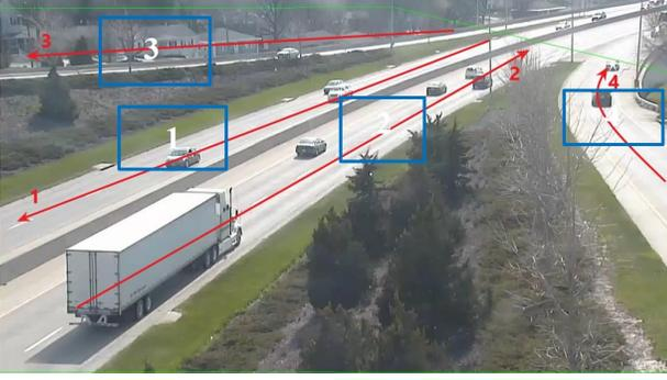
Figure 4. An example of distinguished region tracking. There are 4 regions to monitoring vehicles corresponding with 4 vehicle movements. The red lines are the predefined movements of the scenario.
