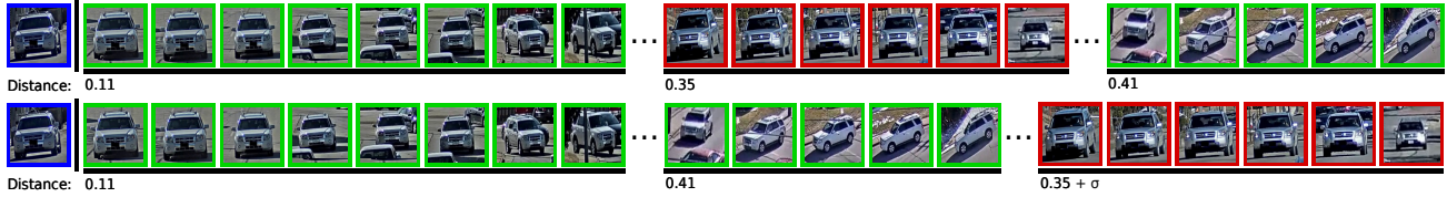
Figure 4. Ranking results before (top) and after (bottom) distance modulation with the orientation information. The blue image is the query, green the positive and red the negative galleries. Images with the same camera view are more likely to have a small distance, therefore we add a constant \sigma to punish them. Images with a very small distance are not punished, see Equation 1
