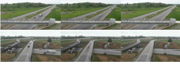
Figure 4. Examples of background modeling. From the left to the right: original frame, background modeling by Moving Average, background modeling by MOG2 ordinally.
