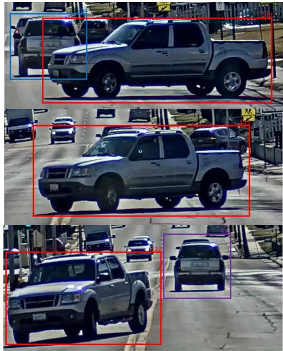
Figure 3: Different from SOT, tracking ID in MOT usually change due to overlapping. Thus, rules, filters or smooth functions is needed.
