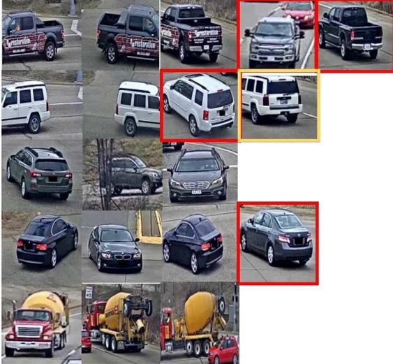
Figure 10: Visualization results of MTMC on five different kinds of vehicles. Each image represents a tracklet and each line represents these tracks from different camera views are classified by MTMC to be from the same vehicle. Yellow box represents false negative and red box represents false positive.
