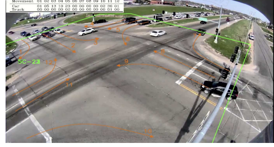
Figure 8. Vehicle counting examples. Orange curves represent for specific movements. Green polygon is an interesting region to do vehicle counting. The table on the top left corner is the counting results of two classes of vehicles counting results in different movements.
