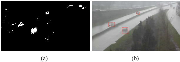
Figure 3. Examples of background subtraction. (a) is related to t'_b , (b) is the final moving object detection results based on background modeling.
