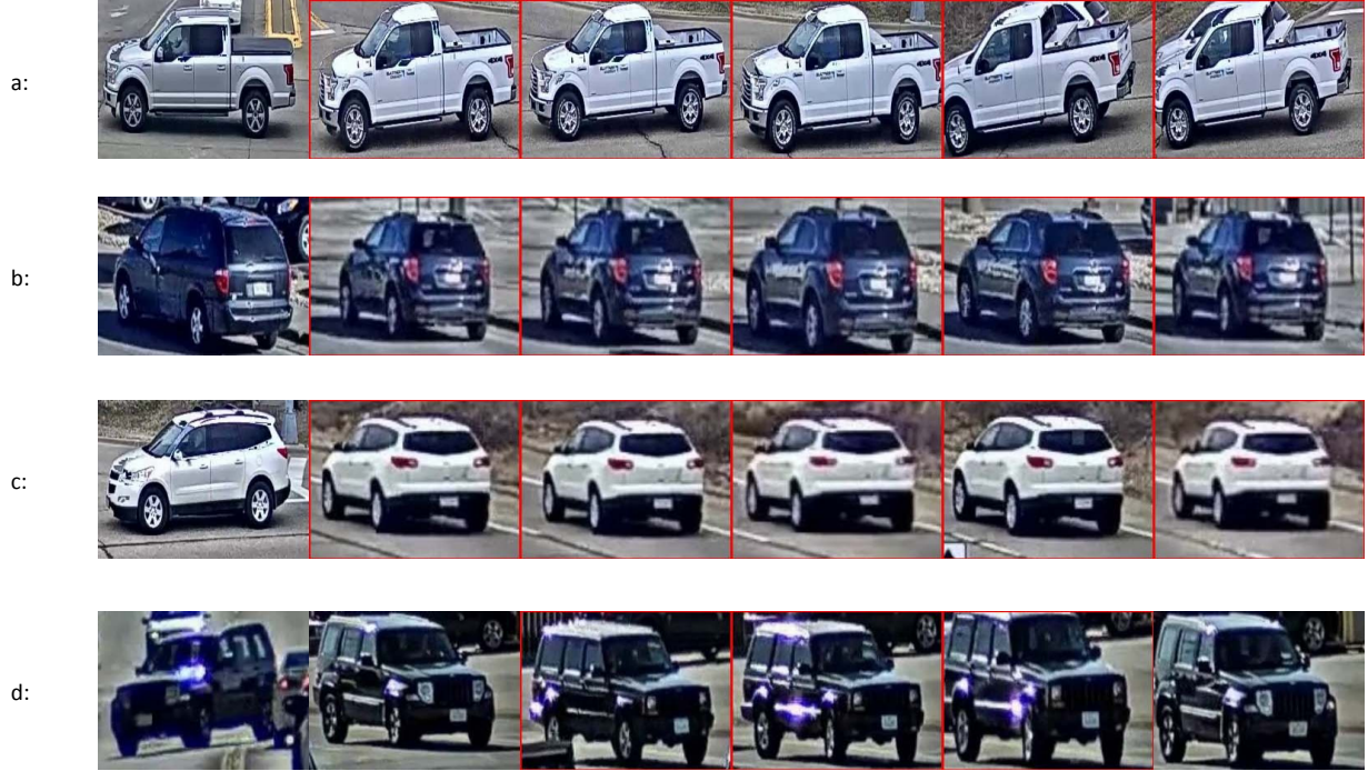
Figure 3. Some false predicts by Vehicle RECT-Net (Red rectangle means the false predicts). As row a and b show: Vehicle RECT-Net usually predicts the vehicle with the similar orientation as the same vehicle ID. As row c and d show: Vehicle RECT-Net usually predicts the vehicle with the similar background as the same vehicle ID.
