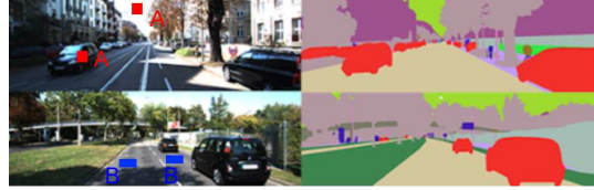
Figure 3. Using semantic knowledge to generate weakly labeled depth. A: the sky is farther than other objects. B: the depth distribution of two road patches should be similar.
