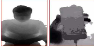
Figure 6. Depth map data helps guarding against presentation attacks. Positive (left) and negative sample (right).
