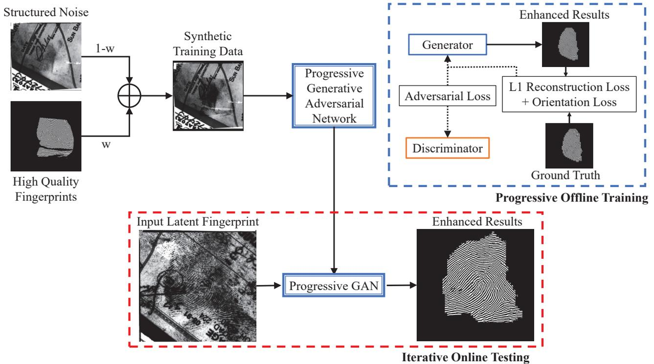
Figure 2. The flowchart of our progressive generative adversarial network based model. Our method can be divided into two stages: Progressive Offline Training (POT) and Iterative Online Testing (IOT). In the POT stage, the dashed lines denote the loss backpropagation path when training our GAN progressively. In IOT stage, the latent fingerprint images are enhanced by the GAN model.
