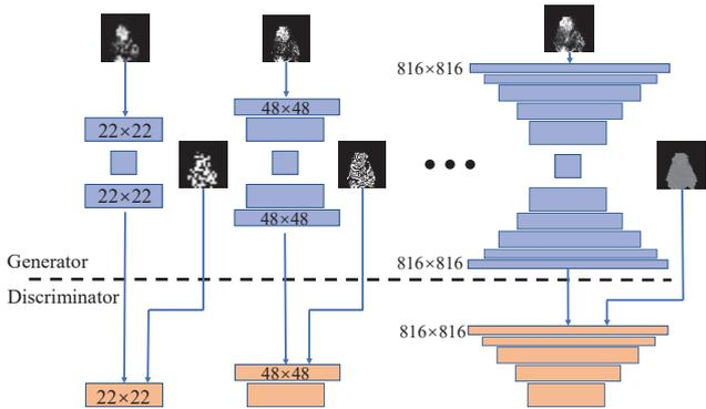
Figure 4. Progressive growing training of GAN. The blue rectangle represents the generator and the orange rectangle represents the discriminator. The training process is from left to right. The number  $N \times N$  in the figure represent the spatial resolution of the input or the output.
