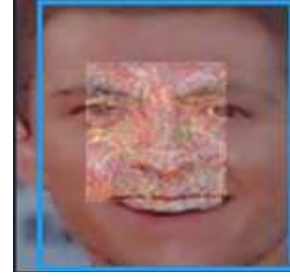
Figure 8: Example of obfuscation attack on the commercial face recognition system in black-box setting. Adversarial light projected on the adversary’s face in the physical domain results in successful obfuscation.
