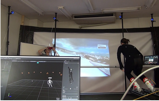
Figure 2. Data capturing of a professional skier on a ski simulator using an eight-camera OptiTrack system.
