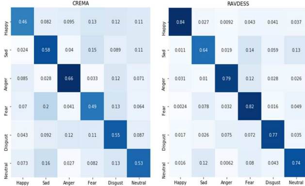
Figure 4: Confusion matrix for AER classification on CREMA and RAVDESS datasets using our methods.
