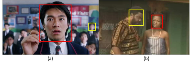
Figure 6. The snapshots with different face sizes and orientations: (a) Face width: 318 pixels (red) vs 63 pixels (yellow); (b) Face orientations: 11° (red) vs 83° (yellow).
