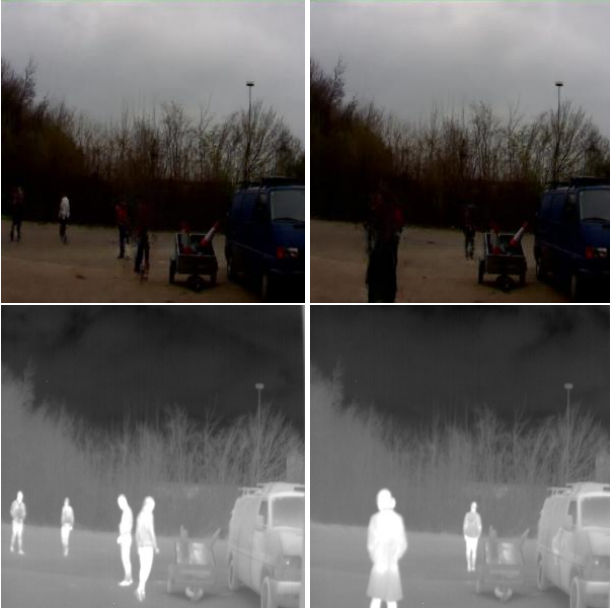
Figure 1: Thales synthetic RGB imagery (top row) translated from real LWIR imagery (bottom row) using our adapted cycleGAN network.
