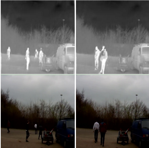
Figure 7: Thales synthetic LWIR imagery (top row) translated from RGB imagery (bottom row).
