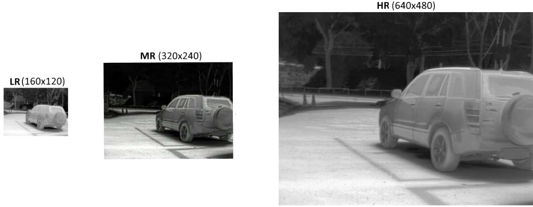
Figure 2. An example of thermal images acquired by each camera. ( left ) LR image with 160 \times 120 native resolution from an Axis Domo P1290. ( middle ) MR image with 320 \times 240 native resolution from an Axis Q2901-E. ( right ) HR image with 640 \times 480 resolution from an FC-6320 FLIR (native resolution is 640 \times 512 ) [10].
