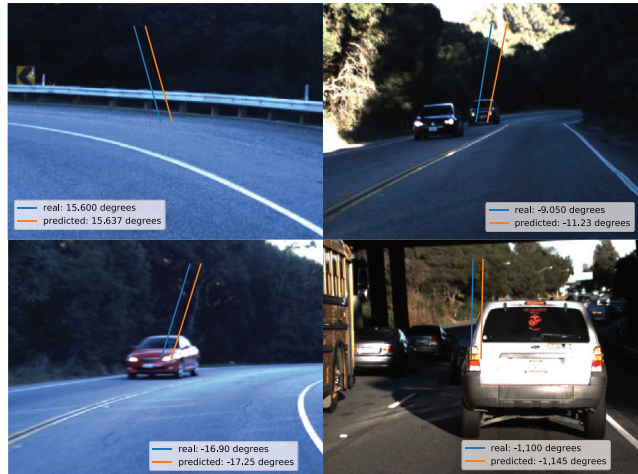
Figure 1. Four frames from the Udacity dataset are shown with their corresponding ground truth (blue) and predicted (orange) steering angles using our Feudal Steering network. The orientation of the lines corresponds to the egocentric steering angle. Our model predicts steering angles within 2.67 degrees of the ground truth angle.
