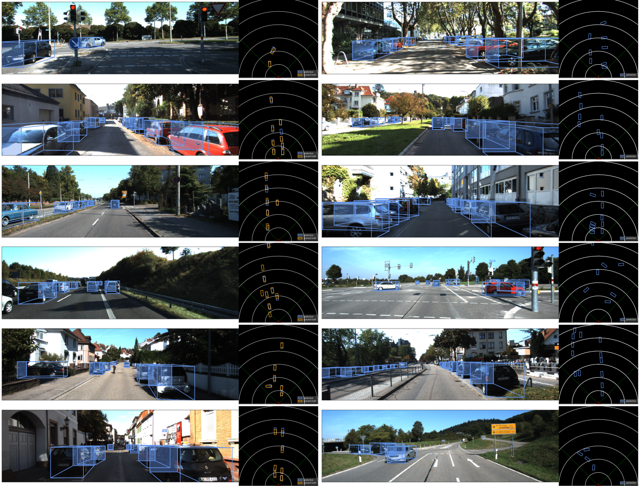
Figure 6. Qualitative examples from the validation (left) and test (right) sets in KITTI. The non-transparent side of the bounding box represents the front part of each car. Bird’s eye view is also provided to show that SMOKE can recover object distances accurately. Note that all these images are not included in the training phase.
