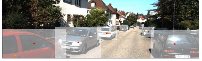
Figure 3. Visualization of difference between 2D center points (red) and 3D projected points (orange). Best viewed in color.
