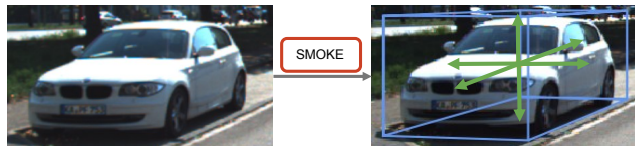
Figure 1. SMOKE directly predicts the 3D projected keypoint and 3D regression parameters on a single image. The whole network is trained end-to-end in a single stage.
