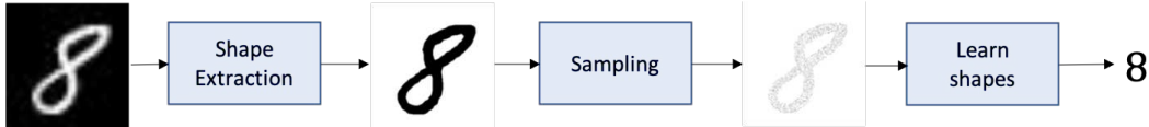
Figure 1: Image shape analysis system. Shape and background in an image are segmented in the shape extraction block, the shape is then sparsely sampled in the sampling block while the learn shapes block learns features characterizing the spatial relationships between the point samples of the shape.
