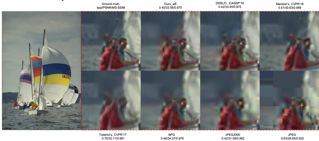
Figure. 3. Kodim09 test result. Note that our model can keep more details than others at the lowest bpp.
